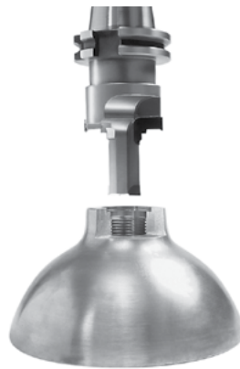
Machining high pressure aluminum cylinders
